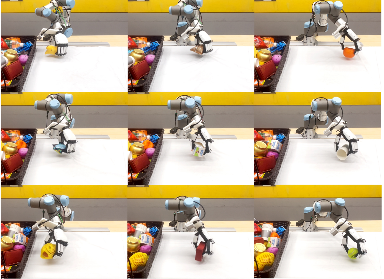
Figure 19 Grasping robustness tested at various spatial locations within the workspace.
