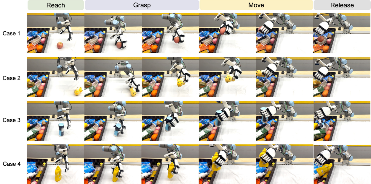
Figure 11 Grasping and placing various objects via end-to-end (arm-hand) VLA policies with a dexterous hand. (See Appendix B for additional real robot tests.)
