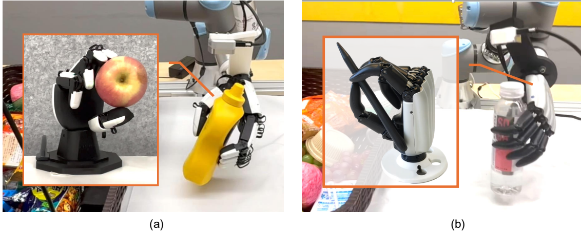
Figure 17 Cross-embodiment validation using two different robotic hands for both the Shared Autonomy framework and the training of end-to-end VLA models: (a) XHAND1 hand [2], and (b) RY-H2 hand [1].
